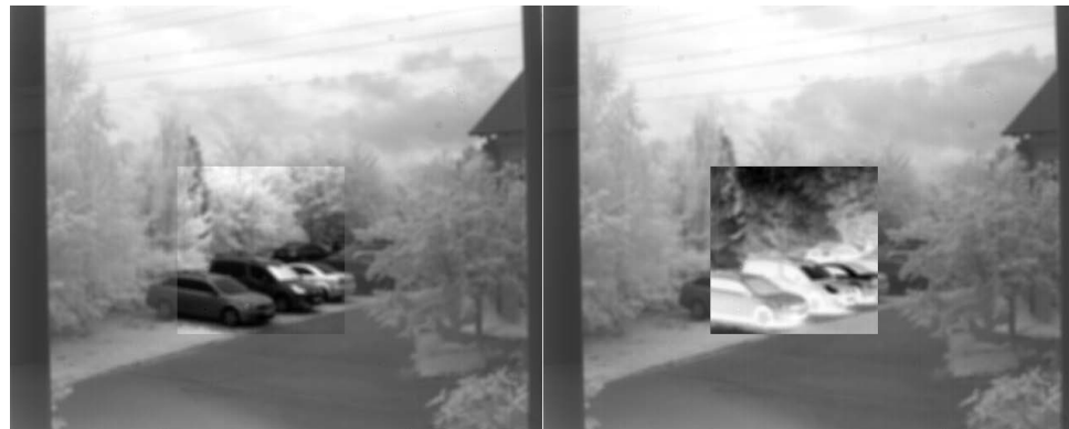
Figure 97: Left: Auto contrast applied to a ROI in the usual way, right: auto contrast with the ContrastAutoIntensity values reversed.
