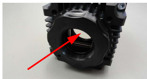
Figure 107: Camera mount without filter, directly exposing the sensor
