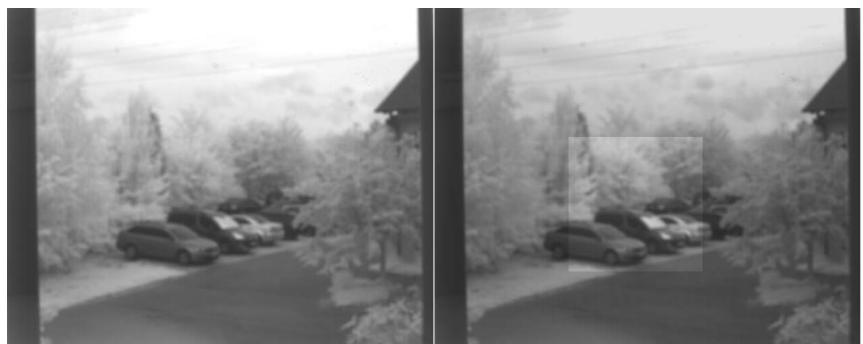
Figure 95: Example for the effect of AutoModeRegionDimOutside. Left: without dimming applied, right: with dimming applied to the outside area.
