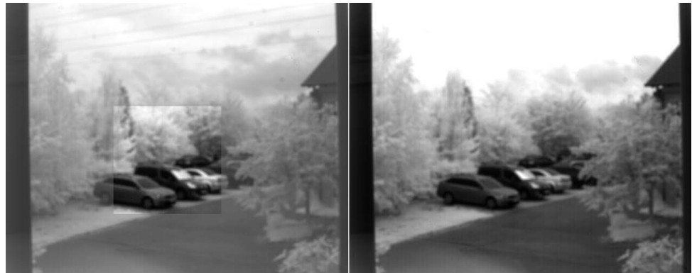
Figure 96: Left: auto contrast applied to ROI, right: auto contrast applied to the whole image.
