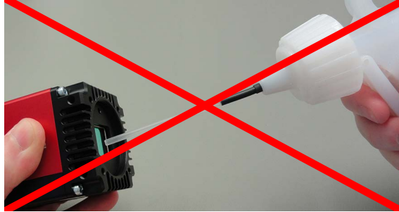
Figure 110: How not to use compressed air
