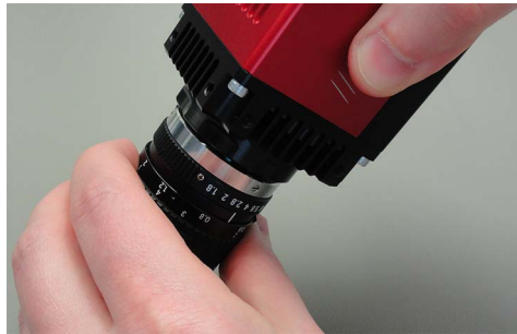
Figure 105: Illustration of camera orientation when removing lens or dust cap
