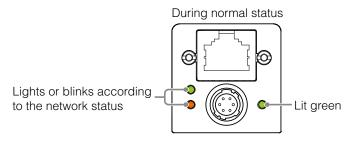
For details on how to read the LEDs, see "LED status and camera status" (page 9) in the "Parts Identification" section.
