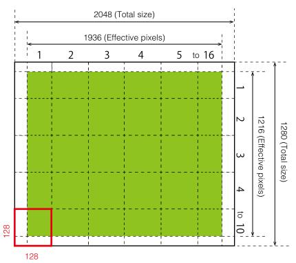
The following shading correction modes are available on the camera. However, as proper interpolation is not performed when ROI settings are configured, execute shading correction at full size before configuring the ROI settings.
