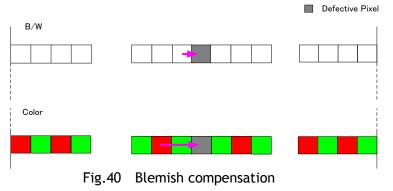
Note: If defective pixels are found consecutively in the horizontal direction, the blemish compensation circuit does not work.
