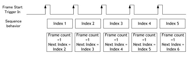
Fig. 31 Behavior of Sequence trigger
