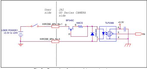
6.3.1 Recommended External Input circuit diagram for customer
