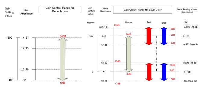
The above drawing shows the relationship between gain setting value (command), gain amplitude, and dB indication. For example, the gain amplitude "x 5.62" equals 15dB.
