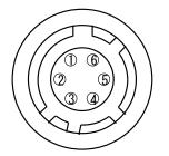
Fig.5 6-pin connector (view from outside)
