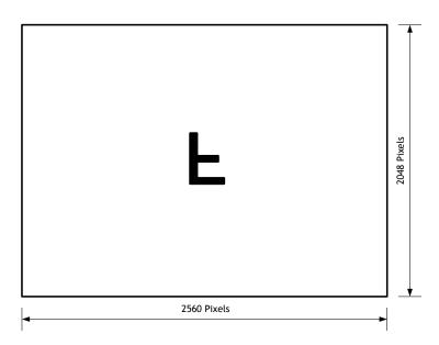
Fig.15 Monochrome sensor layout
