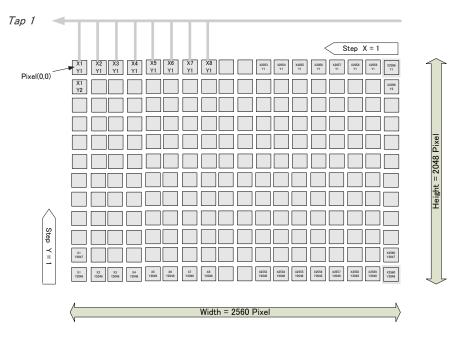
Fig.17 1X - 1Y readout
