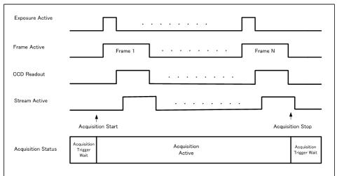
Note: This figure is if the trigger is set to ON, and when the trigger is OFF, FrameActive becomes True at the same timing of AcquisitionActive.
