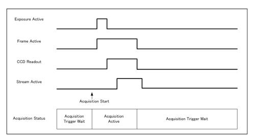
Note: This figure is if the trigger mode is OFF. When the trigger mode is ON, FrameActive becomes True at different AcquisitionActive timing.
