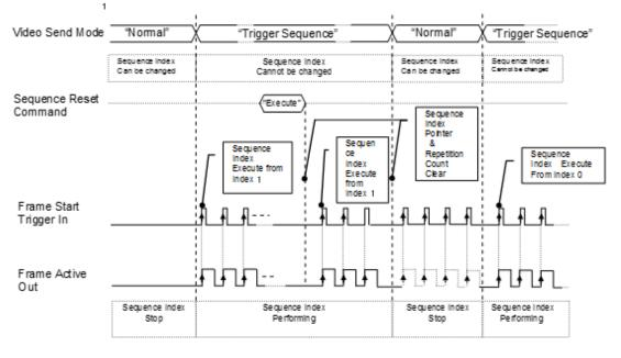
Fig. 32 Behavior if Video Send Mode is set to Trigger Sequence
