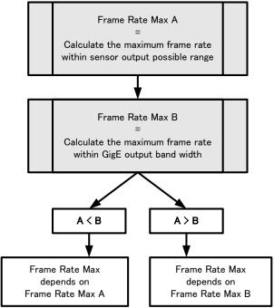
Fig.26 How to determine the maximum frame rate
