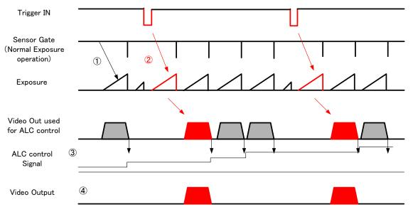
Fig.30 RCT mode timing for ALC operation (Example)
