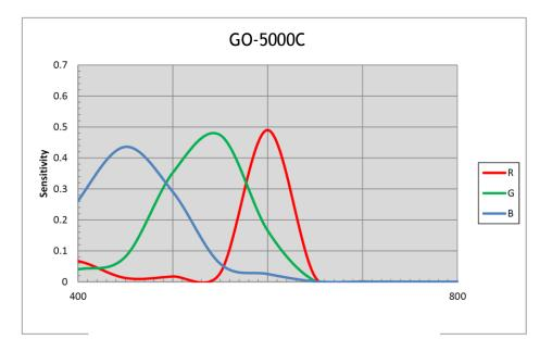
Fig.45 Spectral response (GO-5000C-PGE - with IR Cut Filter)
