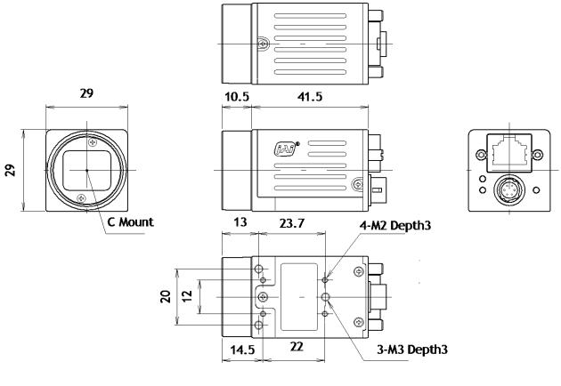
Dimensions tolerance: ± 0.3mm Unit: mm
