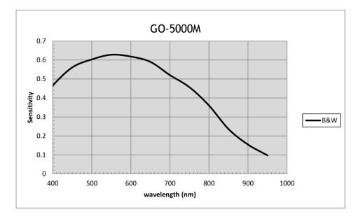
Fig.44 Spectral response (GO-5000M-PGE)
