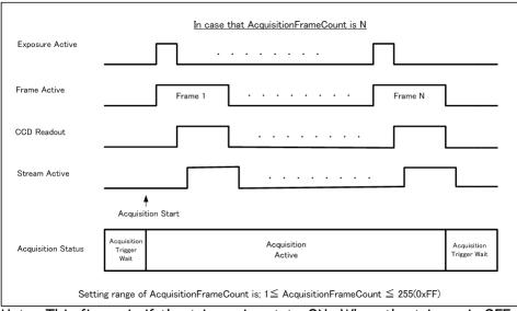
Note: This figure is if the trigger is set to ON. When the trigger is OFF, FrameActive becomes True at the same timing of AcquisitionActive.
