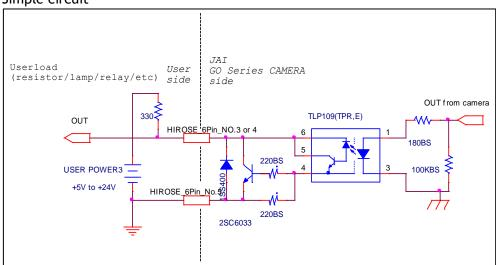
Fig.10 Example of external output circuit(Simple)
