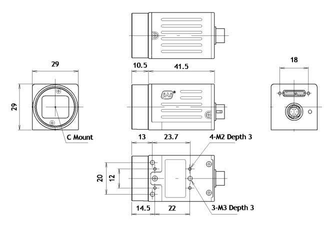
Dimensions tolerance: ± 0.3mm Unit: mm
