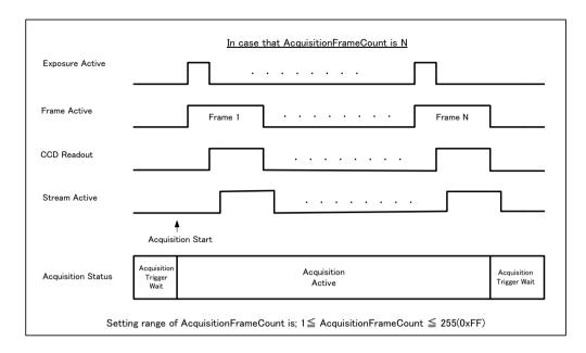
◆ Forcing acquisition to stop While AcquisitionActive is "TRUE", if AcquisitionStop or AcquisitionAbort is initiated, AcquisitionActive becomes "FALSE" (stop capturing). Once the operation is set to "FALSE", the internal FrameCount is reset. However, if AcquisitionStop command is initiated during image output period, AcquisitionActive becomes "FALSE" (stop capturing) after image output is completed. Once, AcquisitionActive becomes "FALSE", the internal count is reset.
