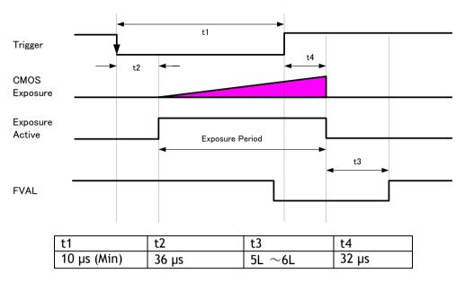
Note 1: The trigger is input through 6P optical input. Accordingly, the timing will be changed if the optical filter is set to the other figures.
