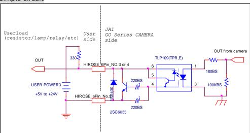
Fig.10 Example of external output circuit(Simple)
