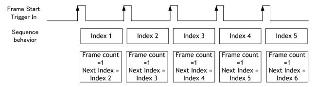
Fig. 27 Behavior of Sequence trigger
