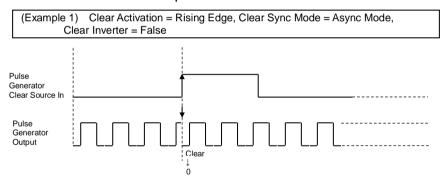
Fig. 12 Counter clear in Async mode
