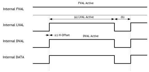
Fig. 17 Horizontal Timing (Vertical timing OFF)
