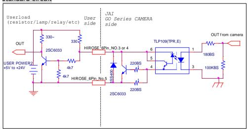
Fig.9 Example of external output circuit(Standard)
