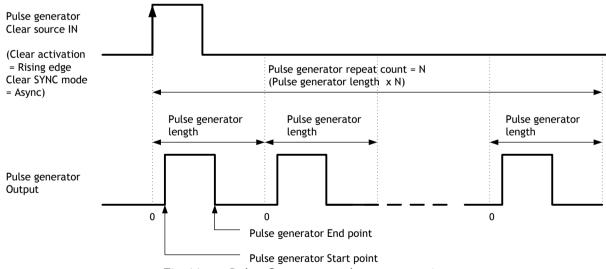
Fig.11 Pulse Generator pulse construction
