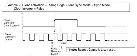
Fig.13 Counter clear in Sync mode
