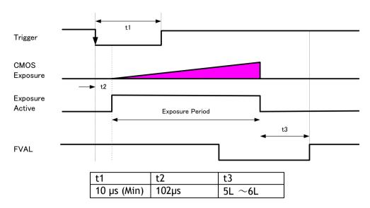
Note 1: The trigger is input through 6P Optical input. Accordingly, the timing will be changed if the optical filter is set to the other figures.
