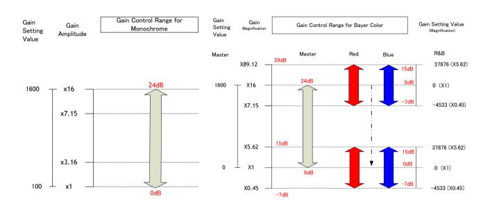
The above drawing shows the relationship between gain setting value (command), gain amplitude, and dB indication. For example, the gain amplitude "x 5.62" equals 15dB.
