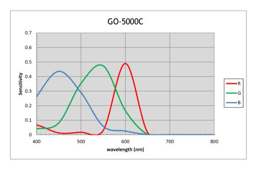
Fig. 42 Spectral response (GO-5000C-USB)
