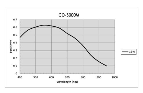
Fig.41 Spectral response (GO-5000M-USB)
