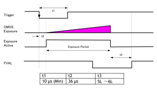
Note 1: The trigger is input through 6P optical input. Accordingly, the timing will be changed if the optical filter is set to the other figures.
