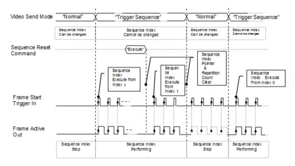
Fig. 28 Behavior if Video Send Mode is set to Trigger Sequence
