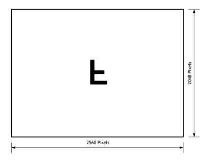
Fig.14 Monochrome sensor layout
