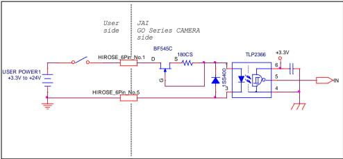
Fig.8 Example of external input circuit
