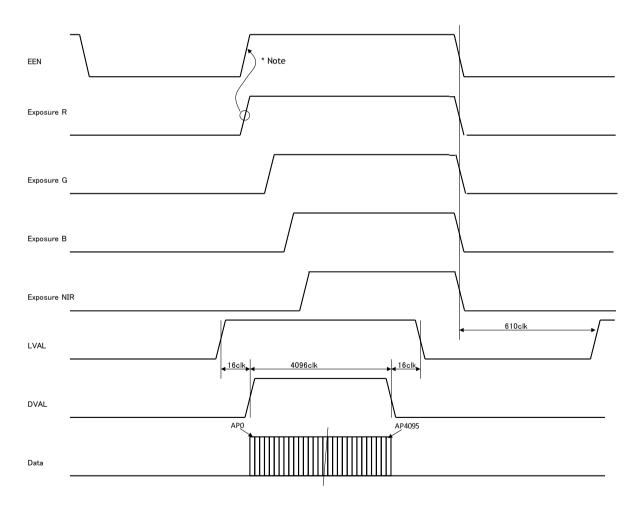
Note: EEN uses channel with the largest exposure value
