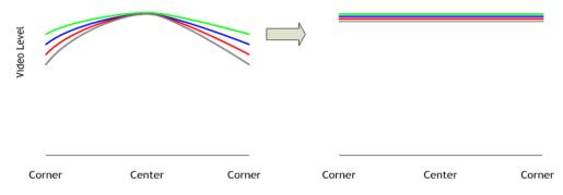
Fig.20 Flat shading correction concept drawing
