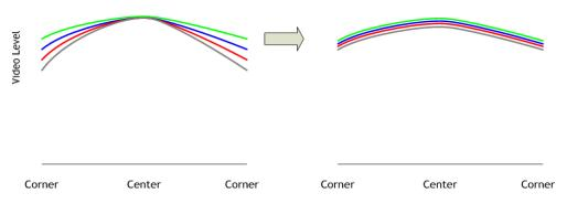
Fig.21 Color shading correction concept drawing
