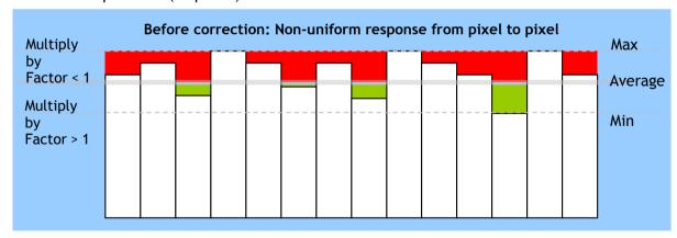
Fig.15 Conceptual drawing for PRNU correction (1)
