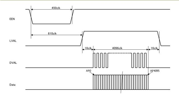
Fig.33 No-Shutter mode / Binning/ Internal
