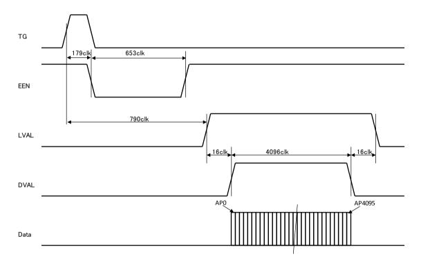
Fig. 35 No-Shutter mode with external trigger
