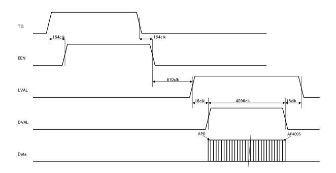
Fig. 44 Pulse Width Control mode
