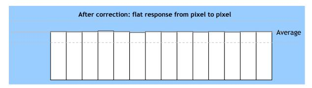
Fig.16 Conceptual drawing for PRNU correction (2)
