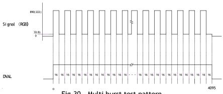
Fig.30 Multi burst test pattern
