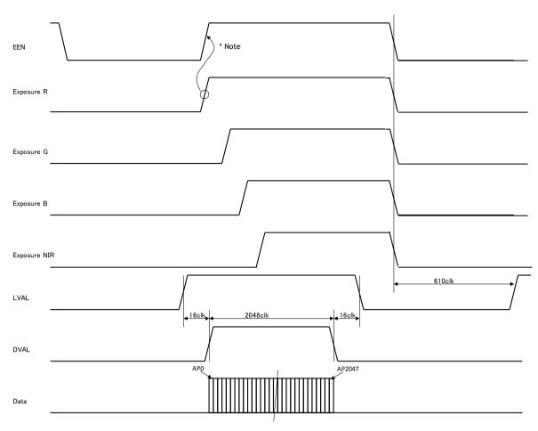
Note: EEN uses channel with the largest exposure value
