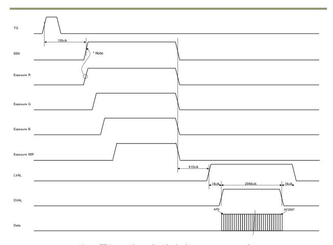
Note: EEN uses channel with the largest exposure value
