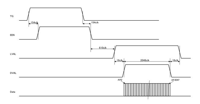
Fig.46 PWC mode /Sub-sampling and Window
