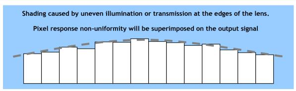
Fig. 19 Shading correction
