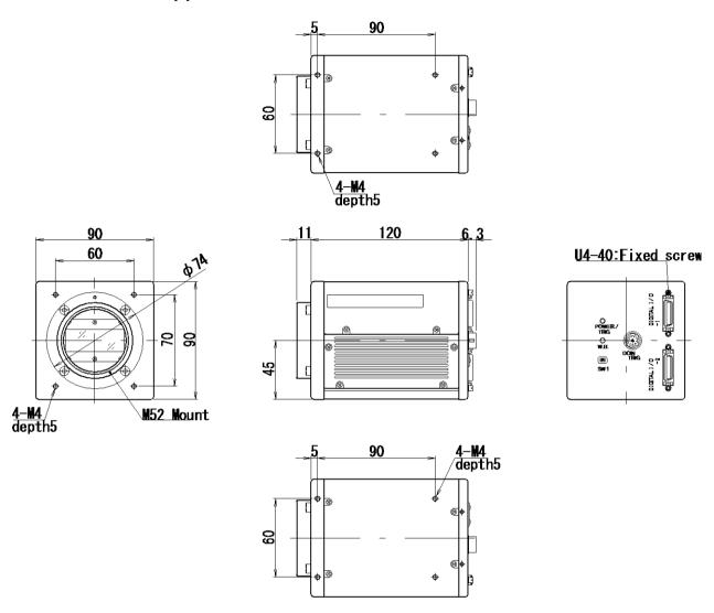
Fig.49 External Appearance and Dimensions (M52 mount)
