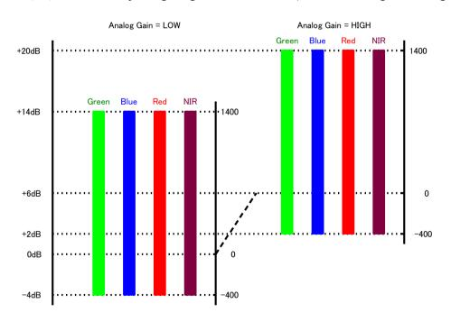
Fig.14 Individual gain mode with gain low and gain high
