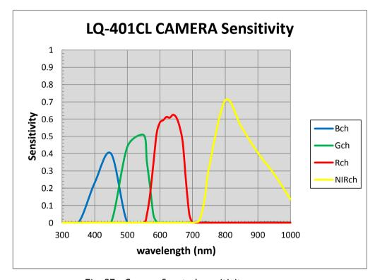
Fig. 27 Camera Spectral sensitivity
