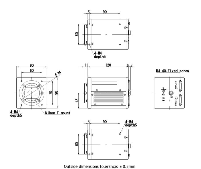
Fig. 50 External Appearance and Dimensions (F mount)
