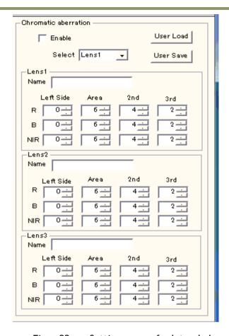
Fig. 22 Setting screen for lateral chromatic aberration
