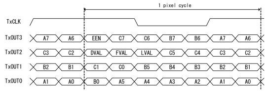
Fig.6 Camera Link output timing
