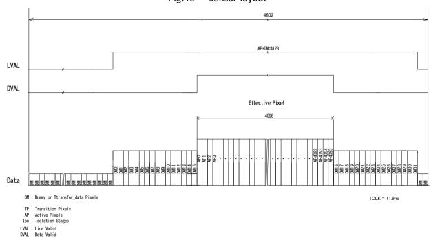
Fig.11 Video output timing
