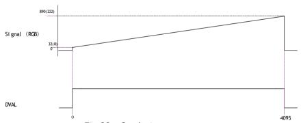
Fig.29 Gradation test pattern
