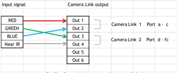
Fig. 7 Camera Link output configuration (Default)
