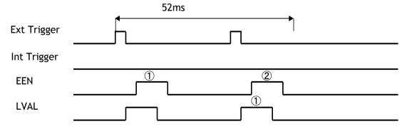
2. If the trigger interval is longer than 52 ms
