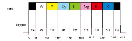
Fig.28 Color bar test pattern
