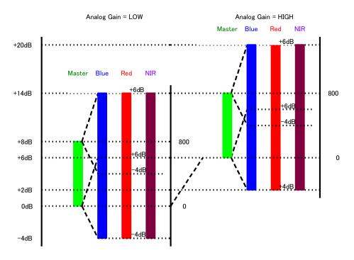
Fig.13 Master gain mode with Gain Low and High
