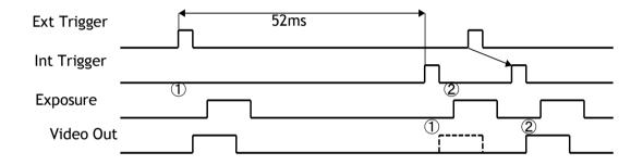
Fig. 48 Auto Interval Timing
