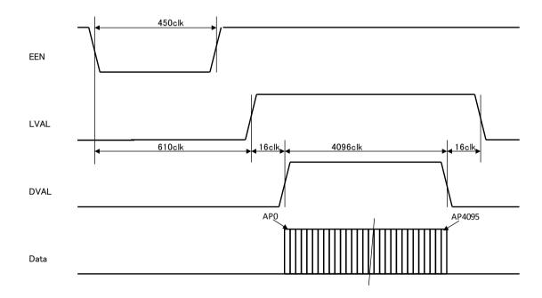
Fig.32 No-Shutter / Internal Trigger mode
