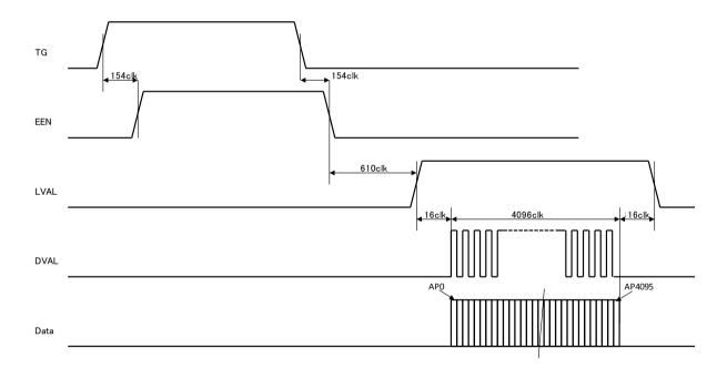
Fig.45 PWC mode /Binning
