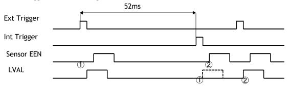
3. If the external trigger timing happens to be the same as the internal trigger timing, the internal trigger is generated again as shown below. In this case, jitter may occur.
