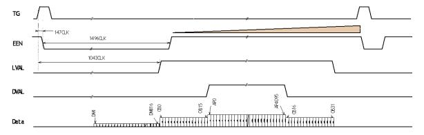
Fig. 33 No-shutter mode with external trigger
