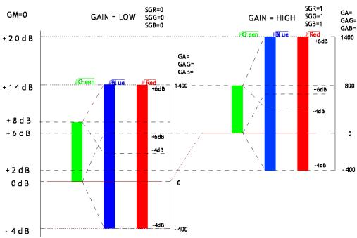
Fig.13 Master gain mode with Gain Low and High
