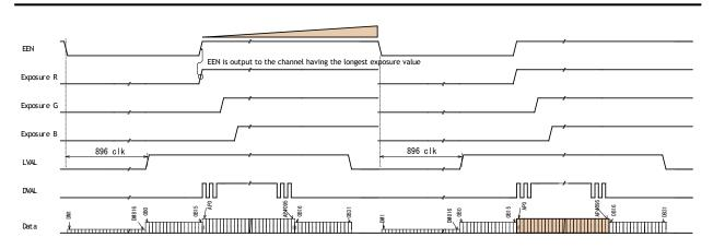
Fig.37 Shutter-select mode / Binning / Internal
