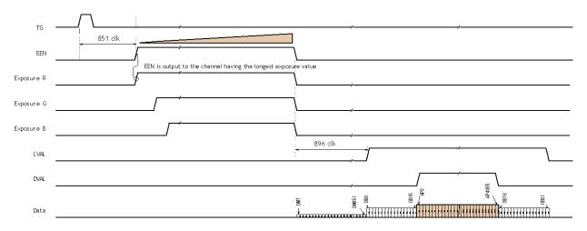
Fig. 39 Shutter-select mode with external trigger (and individual exposure)
