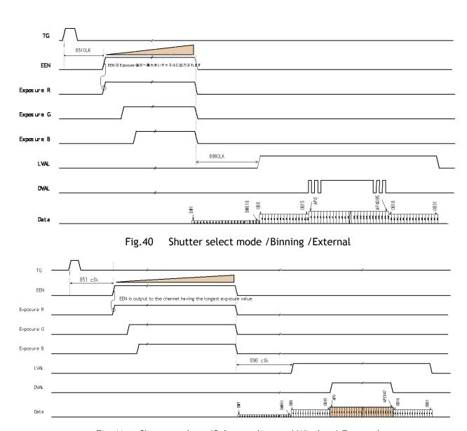
Fig.41 Shutter-select /Sub-sampling and Window/ External
