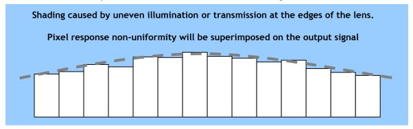
Fig. 20 Shading correction
