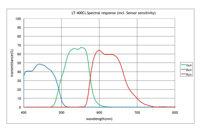
Fig.34 Spectral response including prism and sensors
