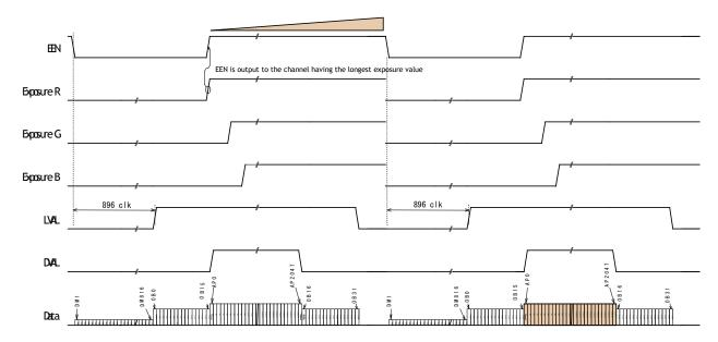
Fig.38 Shutter -select mode/Sub-sampling and Window/ Internal
