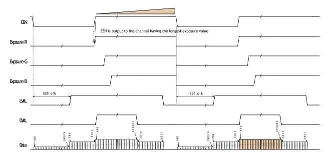
Fig. 36 Shutter-select mode with internal line rate generator (and individual exposure)
