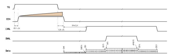
Fig. 42 Pulse Width Control mode
