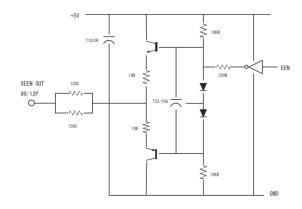
Fig. 7 XEEN Circuit (12-pin Hirose)
