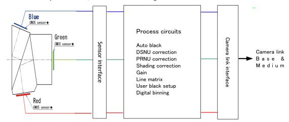
Fig.8 Sensor block diagram
