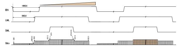
Fig. 30 No-shutter / internal trigger mode
