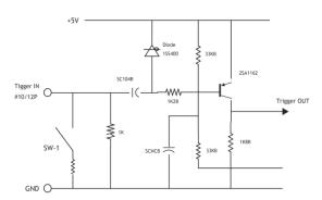
Fig. 6 Trigger input (12-pin Hirose)
