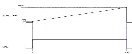
Fig.25 Gradation test pattern
