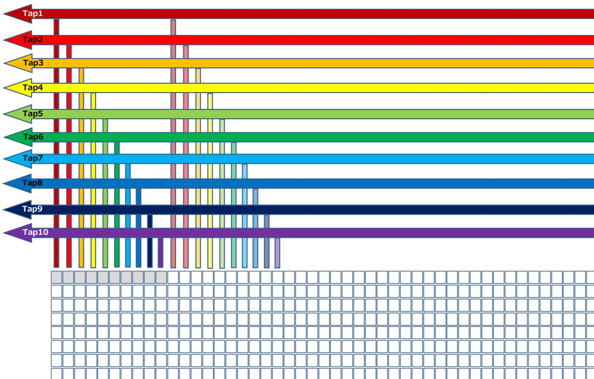
In one cycle, the data of ten pixels is output via Camera Link.
