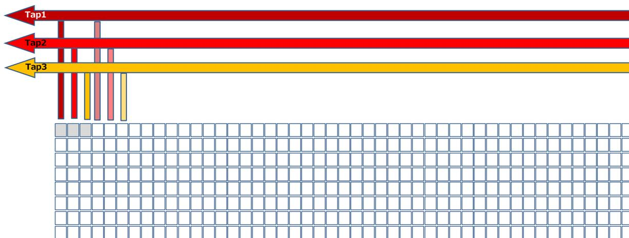
In one cycle, the data of three pixels is output via Camera Link.
