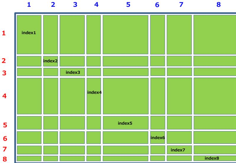
You can set the readout area by setting [SensorMultiRoiHorizontalEnable] and [SensorMultiRoiVerticalEnable] of index 1 to 8 to True.
