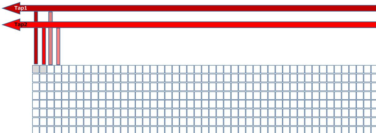
In one cycle, the data of two pixels is output via Camera Link.
