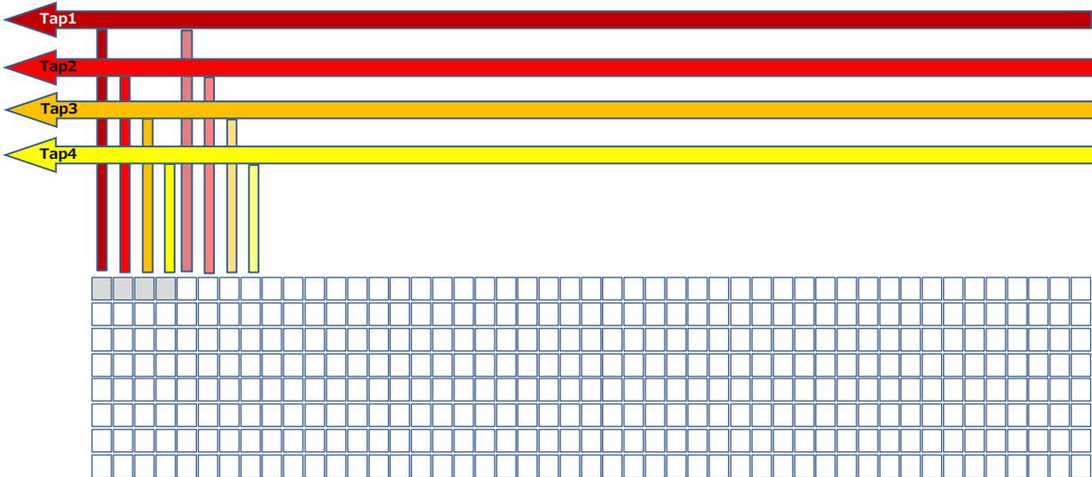
In one cycle, the data of four pixels is output via Camera Link.
