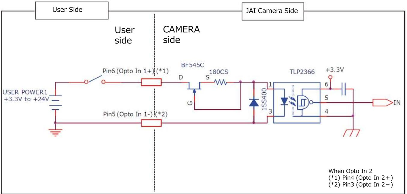
**Recommended external output circuit diagram (reference example)**
