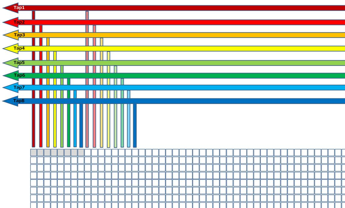
In one cycle, the data of eight pixels is output via Camera Link.
