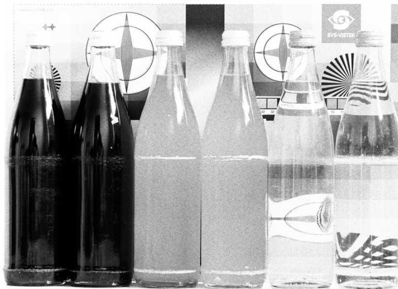
Fig.: 6-1: Noise caused by too much gain
