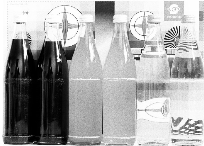
Fig.: 5-1: Noise caused by too much gain
