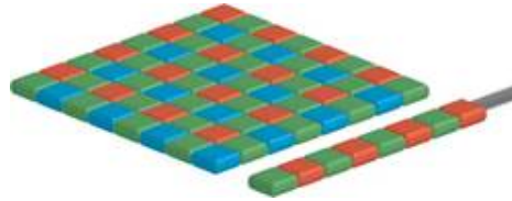
Fig.: 5-3: Sensor with Bayer pattern
