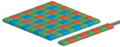
Fig.: 5-3: Sensor with Bayer pattern
