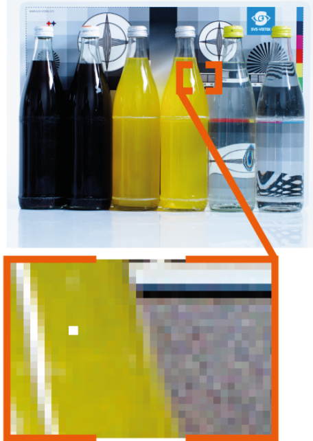
Fig.: 5-20: Illustration of a defect pixel
