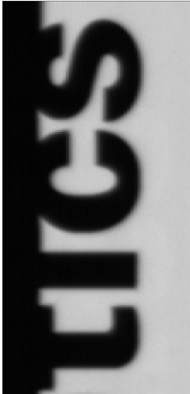
30° Camera Angle, 8k Camera, 80 mm lens, 20 \mu\text{m} Object Pixel, Spatial Correction =9.2, No Parallax Correction
