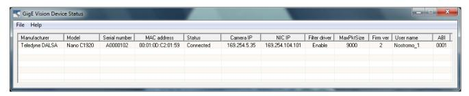
In the event that the device is physically connected, but the Sapera GigE Server icon is indicating that the connected device is not recognized, click Scan Network to restart the discovery process. Note that the GigE server periodically scans the network automatically to refresh its state. See Troubleshooting for network problems.
