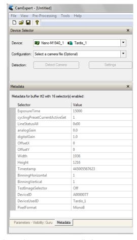
Alternatively, Sapera LT provides a demo program called GigEMetaDataDemo.exe which will grab a number of frames and display the metadata or save it to a file (.csv). In addition, source code and C++ project files are included for a console based executable.
