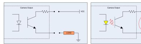
Examples of Logic HI and Logic LO output circuits
