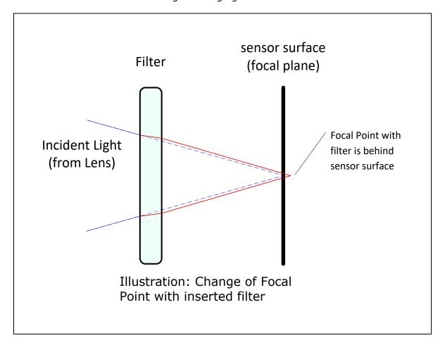
In this example when a glass filter is inserted between the lens and the camera sensor, the focal point is now about 1/3 of the filter thickness behind the sensor plane. Genie Nano-5G filters are specified as 1mm thick.
