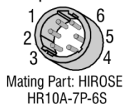
Figure 12: 6-pin Hirose Circular Male Power Plug—Power Connector
