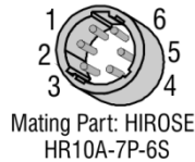
Figure 8: 6-pin Hirose Circular Male Power Plug—Power Connector
