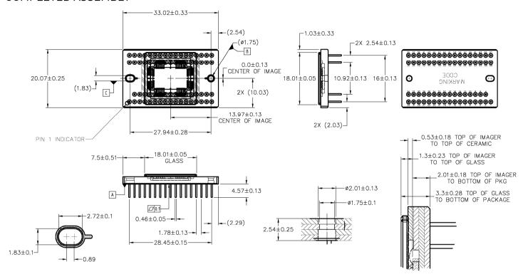
Figure 21: Completed Assembly
