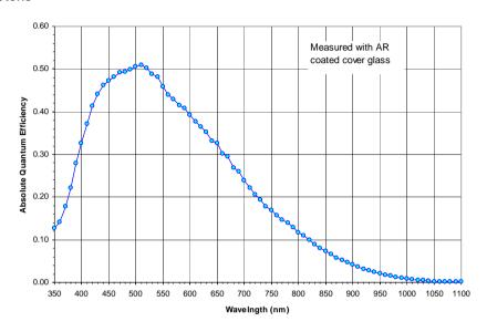
Figure 3: Monochrome with Microlens Quantum Efficiency
