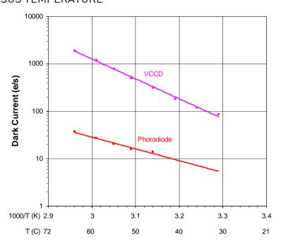
Figure 7: Dark Current versus Temperature
