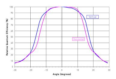
Figure 6: Monochrome with Microlens Angular Quantum Efficiency
