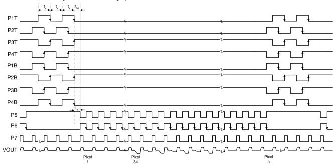
Figure 20: Line and Pixel Timing - Vertical Binning by 2
