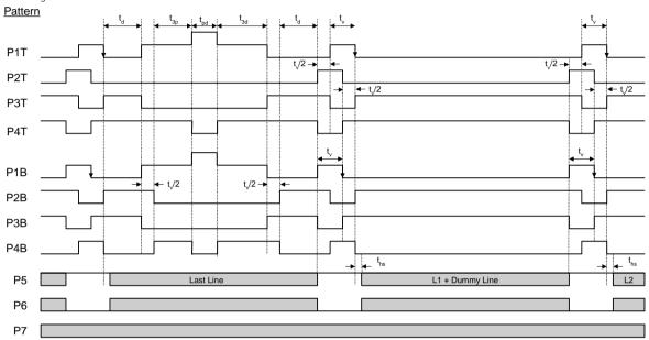
Figure 15: Photodiode Transfer Timing
