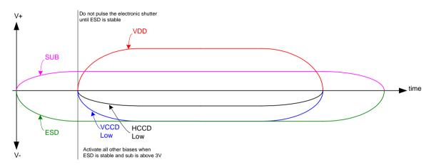
Figure 12: Power Up and Power Down Sequence
