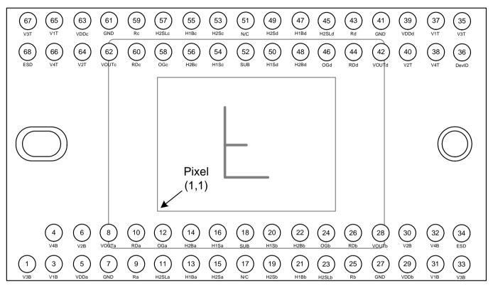
Figure 2: Package Pin Designations - Top View
