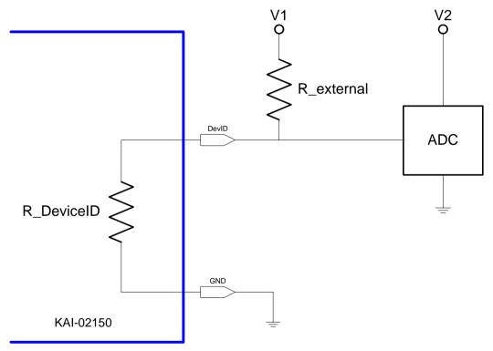
Figure 14: Device Identification Recommended Circuit
