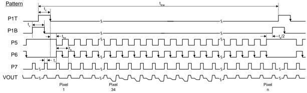
Figure 16: Line and Pixel Timing
