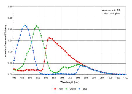
Figure 5: Color with Microlens Quantum Efficiency
