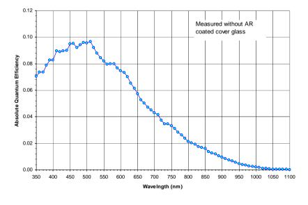
Figure 4: Monochrome without Microlens Quantum Efficiency
