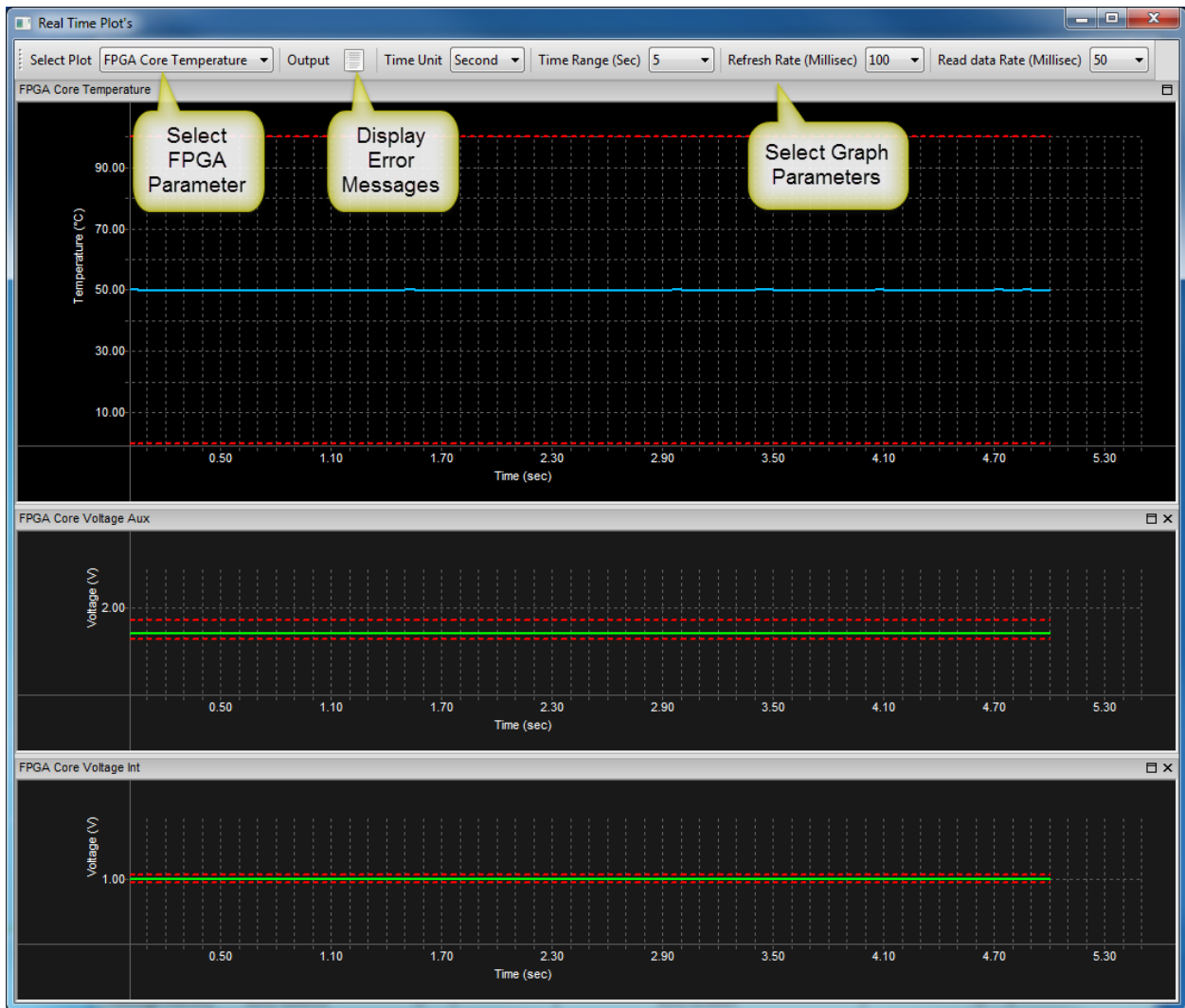
Figure 13: Diagnostic Tool Live Monitoring Window
