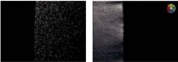
Detecting the separation between two black materials. The fabric on the left reflects infrared light, while the fabric on the right absorbs infrared light, creating contrast.
