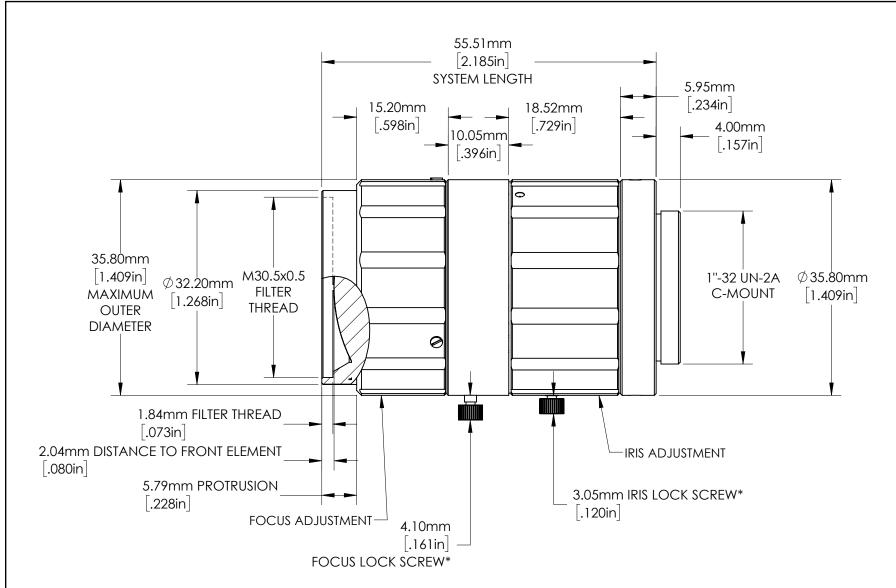
VIEW OF LENS FOCUSED TO 250mm WORKING DISTANCE
