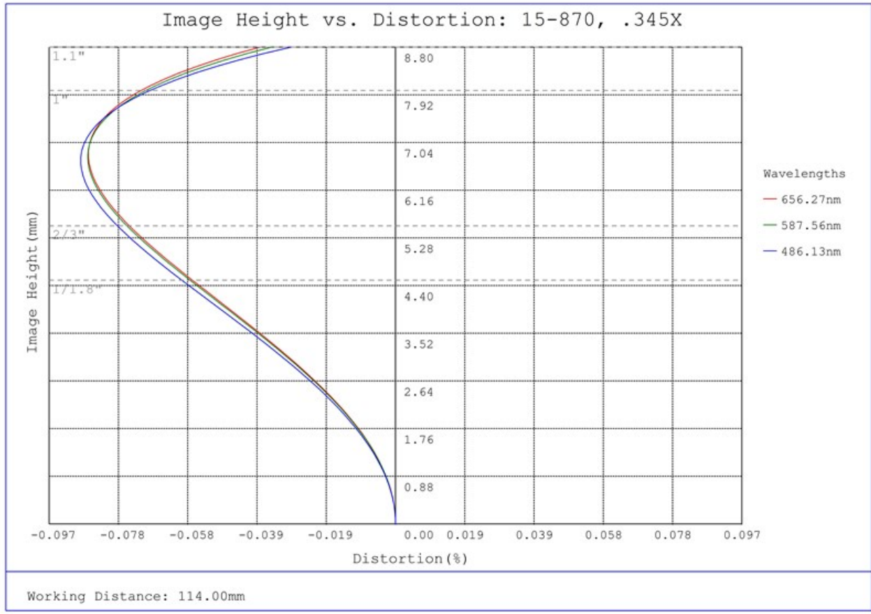
#15-870, 0.345X CobaltTTL Telecentric Lens, Distortion Plot
