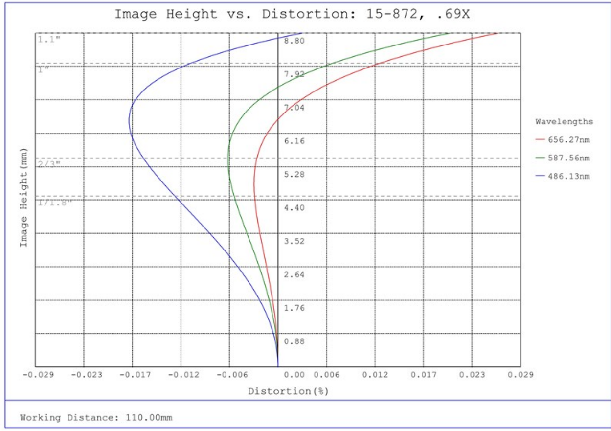
#15-872, 0.69X CobaltTL Telecentric Lens, Distortion Plot
