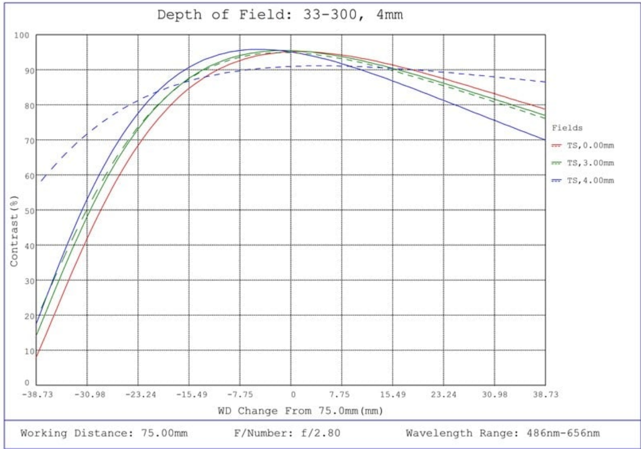
#33-300, 4mm UC Series Fixed Focal Length Lens, Depth of Field Plot, 75mm Working Distance, f2.8
