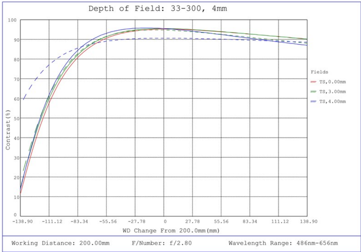
#33-300, 4mm UC Series Fixed Focal Length Lens, Depth of Field Plot, 200mm Working Distance, f2.8
