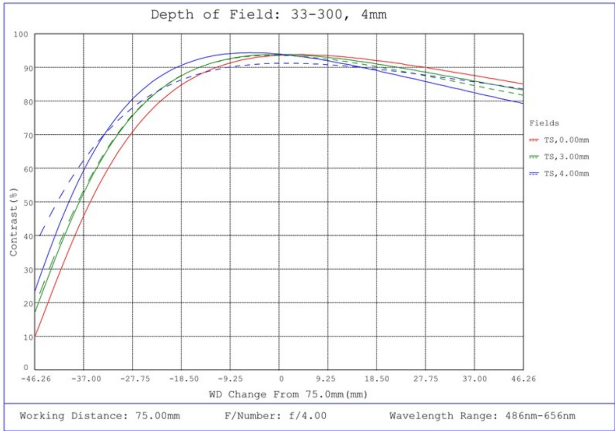
#33-300, 4mm UC Series Fixed Focal Length Lens, Depth of Field Plot, 75mm Working Distance, f4
