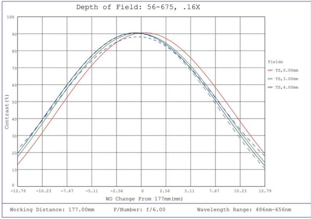
#56-675, 0.16X SilverTL™ Telecentric Lens, Depth of Field Plot, 177mm Working Distance, f6
