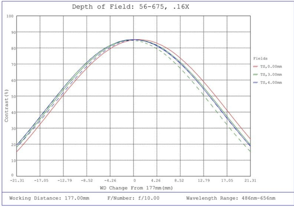
#56-675, 0.16X SilverTL™ Telecentric Lens, Depth of Field Plot, 177mm Working Distance, f10
