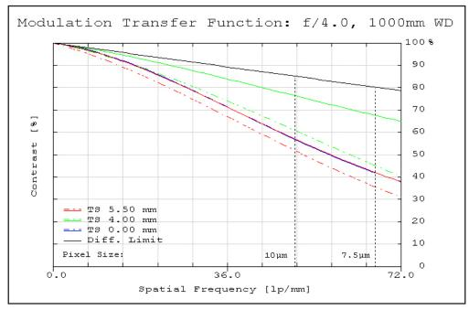
Figure 9: Image space polychromatic diffraction FFT Modulation Transfer Function (MTF) for  $\lambda = 486$ nm to 656nm. Included are Tangential and Sagittal values for field points on center, at 70% of full field and at the maximum sensor format. Solid black line indicates diffraction limit determined by f/#-defined aperture. Frequencies corresponding to the Nyquist resolution limit of pixel sizes are indicated.
