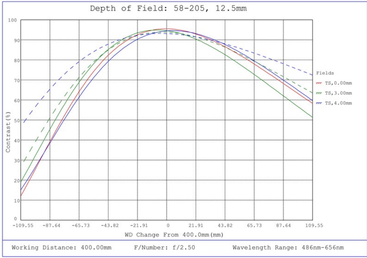
#58-205, 12.5mm FL f/2.5, Blue Series M12 Lens, Depth of Field Plot, 400mm Working Distance, f2.5
