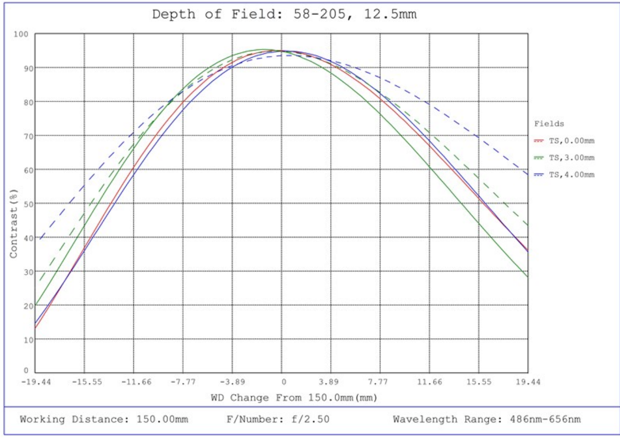
#58-205, 12.5mm FL f/2.5, Blue Series M12 Lens, Depth of Field Plot, 150mm Working Distance, f2.5
