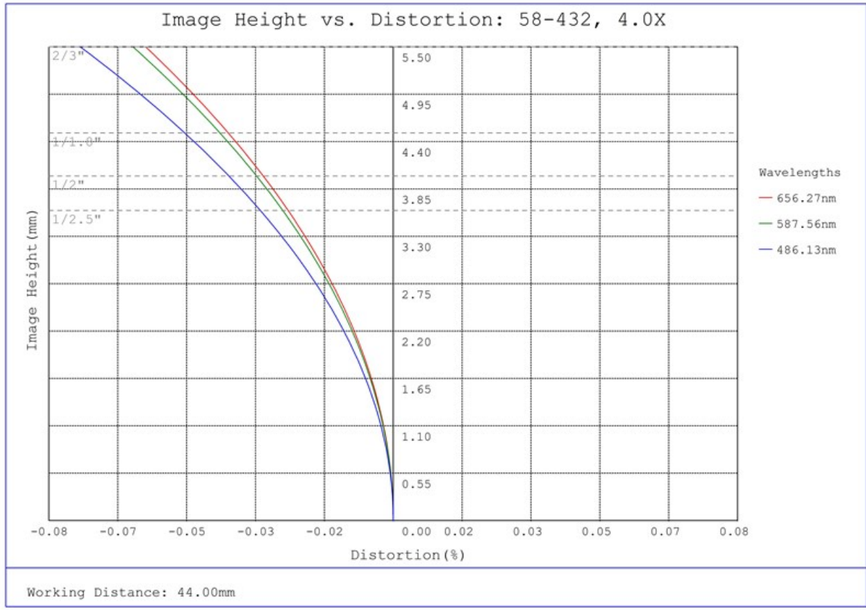
#58-432, 4.0X SilverTL™ Telecentric Lens, Distortion Plot
