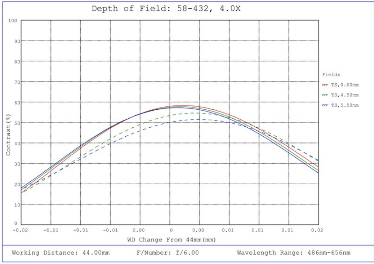
#58-432, 4.0X SilverTL™ Telecentric Lens, Depth of Field Plot, 44mm Working Distance, f6
