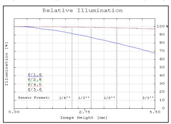
Figure 2: Relative illumination (center to corner)
