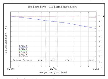
Figure 2: Relative illumination (center to corner)
