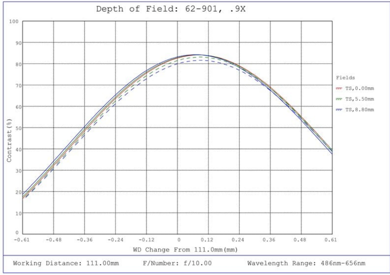
#62-901, 0.9X CobaltTL Telecentric Lens, Depth of Field Plot, 111mm Working Distance, f10
