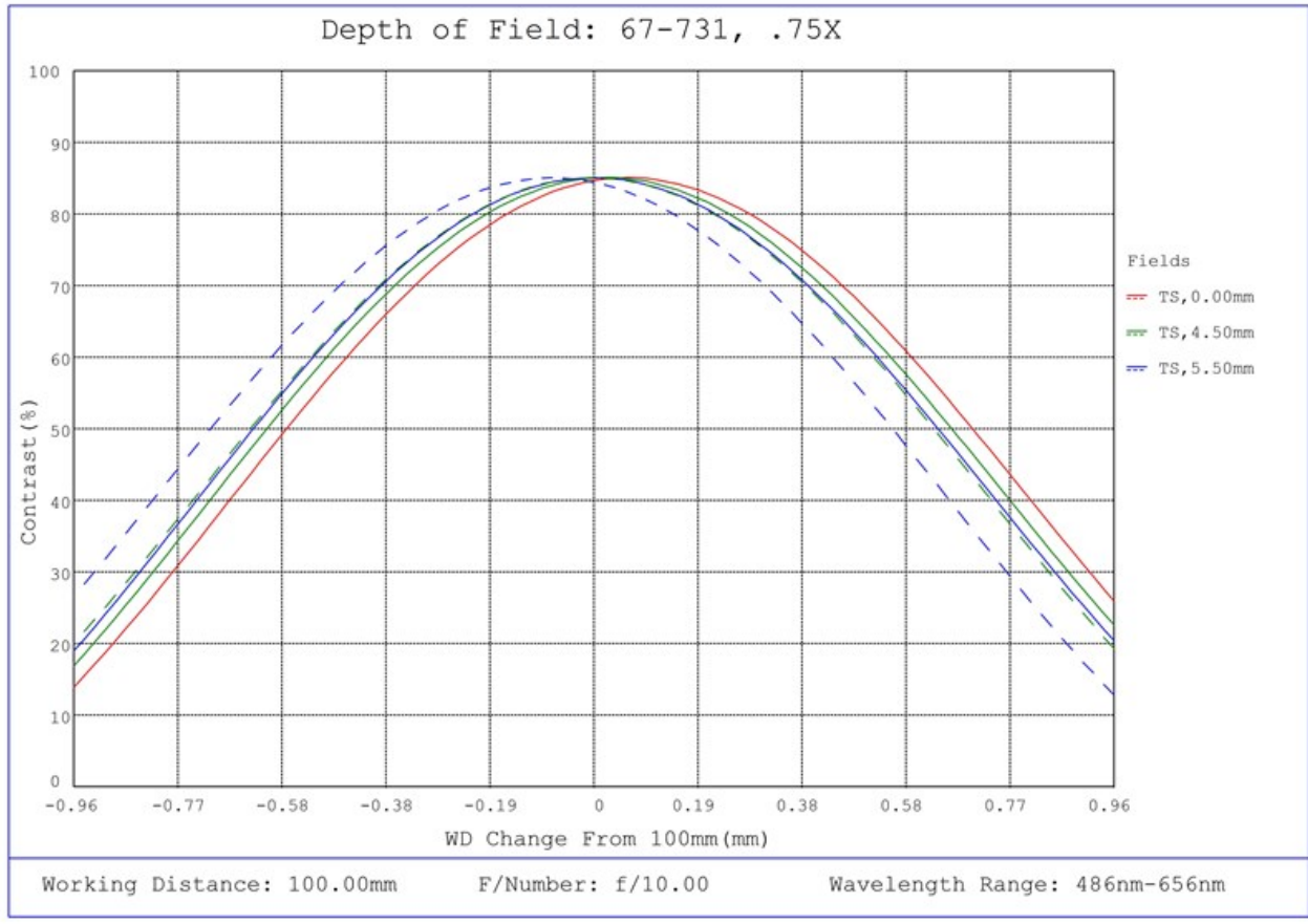
#67-731, 0.75X SilverTL™ Telecentric Lens, Depth of Field Plot, 100mm Working Distance, f10
