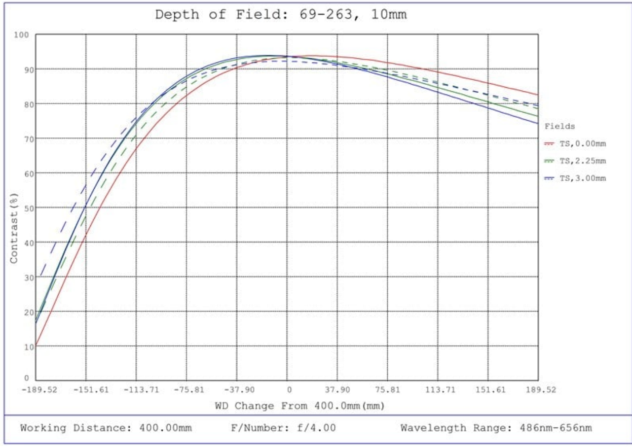
#69-263, 10mm FL f/4, Blue Series M12 Lens, Depth of Field Plot, 400mm Working Distance, f4
