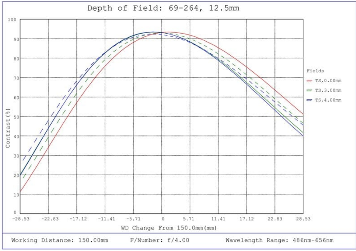
#69-264, 12.5mm FL f/4, Blue Series M12 Lens, Depth of Field Plot, 150mm Working Distance, f4
