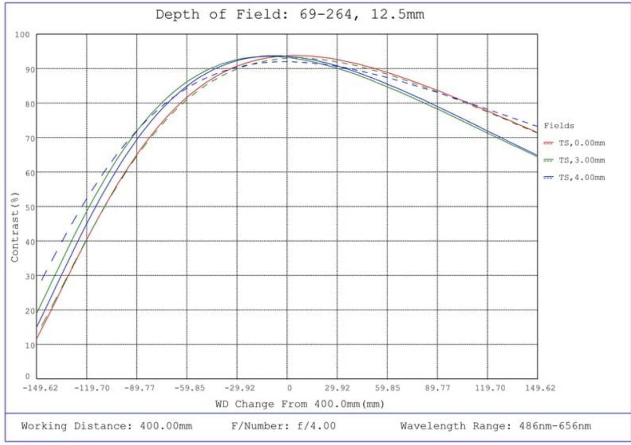
#69-264, 12.5mm FL f/4, Blue Series M12 Lens, Depth of Field Plot, 400mm Working Distance, f4
