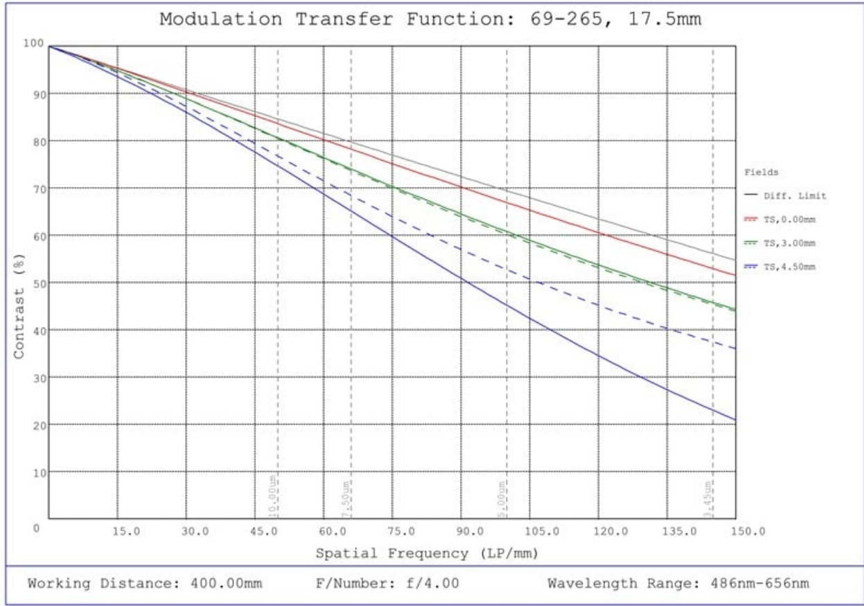
#69-265, 17.5mm FL f/4, Blue Series M12 Lens, Modulated Transfer Function (MTF) Plot, 400mm Working Distance, f4
