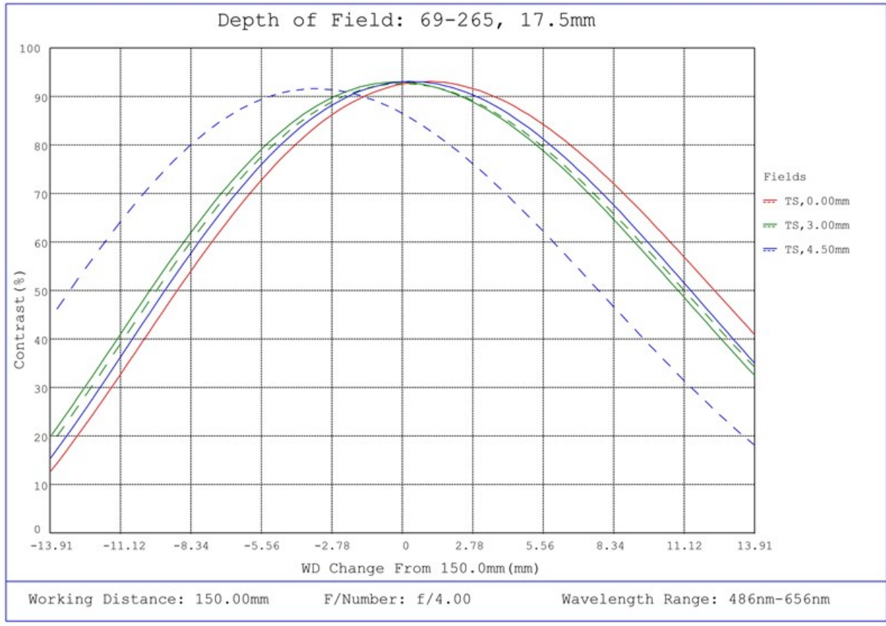
#69-265, 17.5mm FL f/4, Blue Series M12 Lens, Depth of Field Plot, 150mm Working Distance, f4
