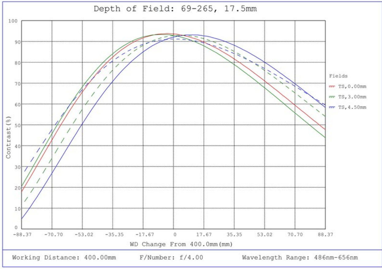
#69-265, 17.5mm FL f/4, Blue Series M12 Lens, Depth of Field Plot, 400mm Working Distance, f4
