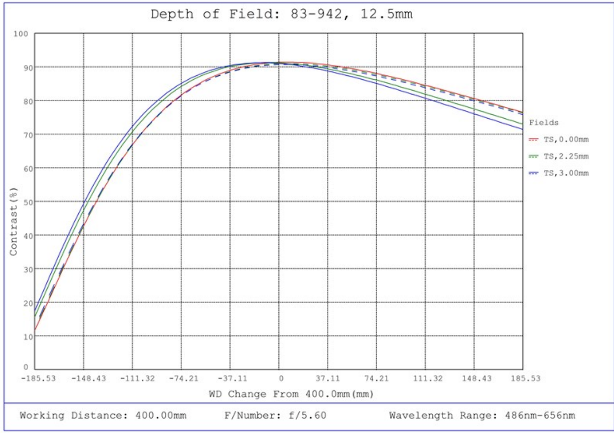
#83-942, 12.5mm FL f/5.6, Blue Series M12 Lens, Depth of Field Plot, 400mm Working Distance, f5.6
