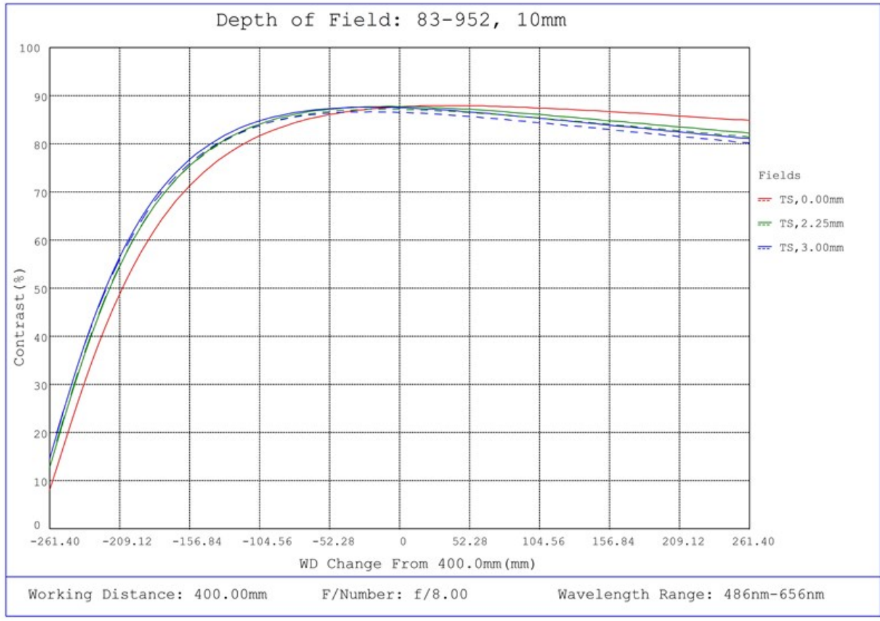
#83-952, 10mm FL f/8, Blue Series M12 Lens, Depth of Field Plot, 400mm Working Distance, f8
