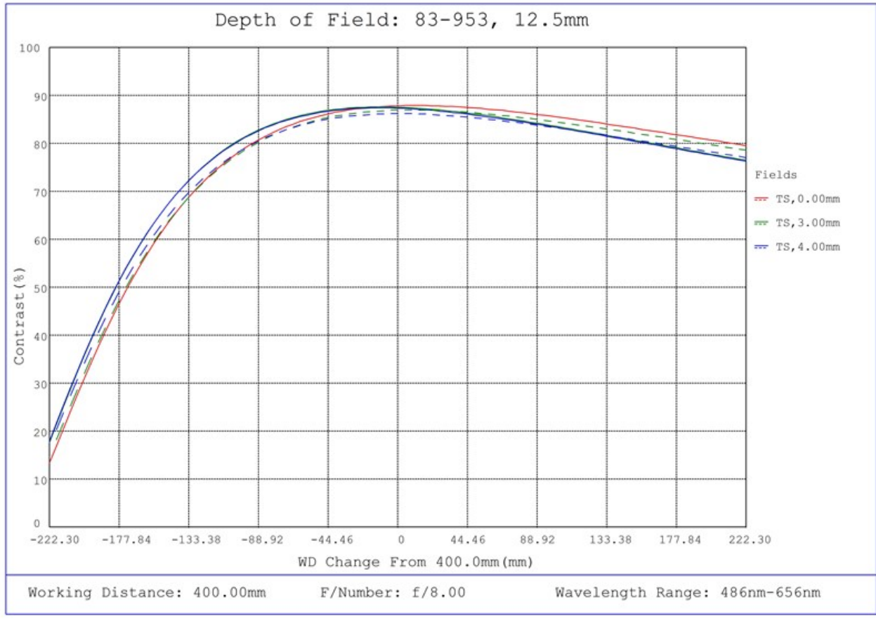
#83-953, 12.5mm FL f/8, Blue Series M12 Lens, Depth of Field Plot, 400mm Working Distance, f8
