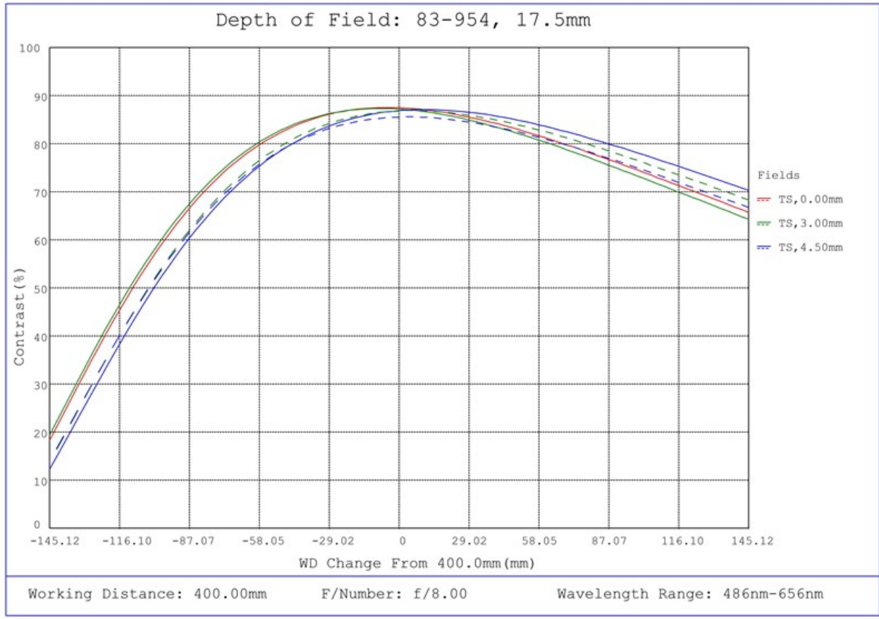
#83-954, 17.5mm FL f/8, Blue Series M12 Lens, Depth of Field Plot, 400mm Working Distance, f8
