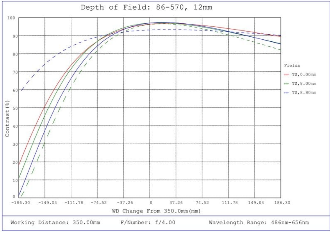
#86-570, 12mm Focal Length, HP Series Fixed Focal Length Lens, Depth of Field Plot, 350mm Working Distance, f4
