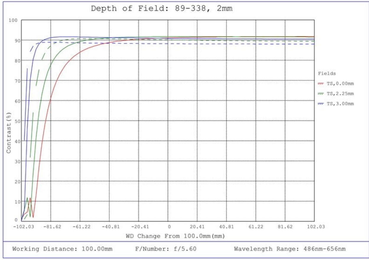
#89-338, 2mm FL f/5.6, Blue Series M12 Lens, Depth of Field Plot, 100mm Working Distance, f5.6
