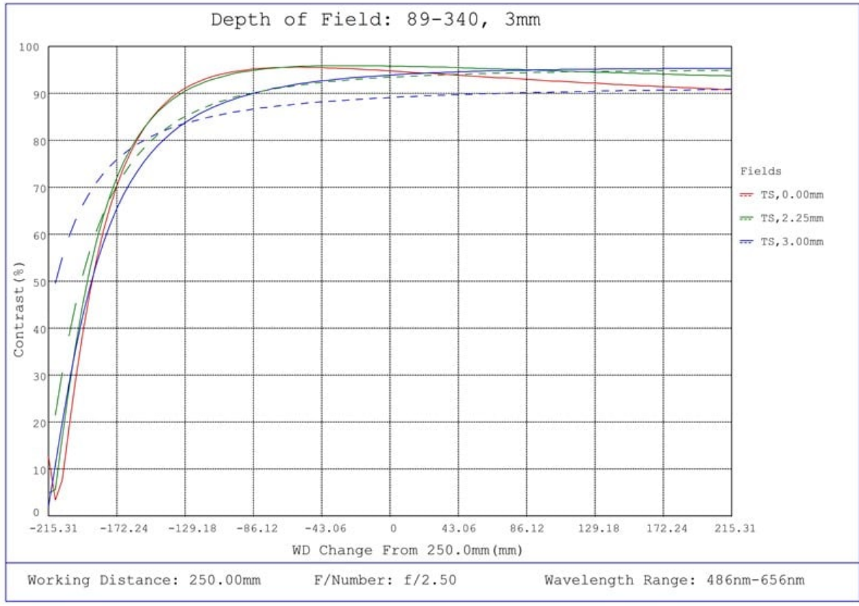
#89-340, 3mm FL f/2.5, Blue Series M12 Lens, Depth of Field Plot, 250mm Working Distance, f2.5
