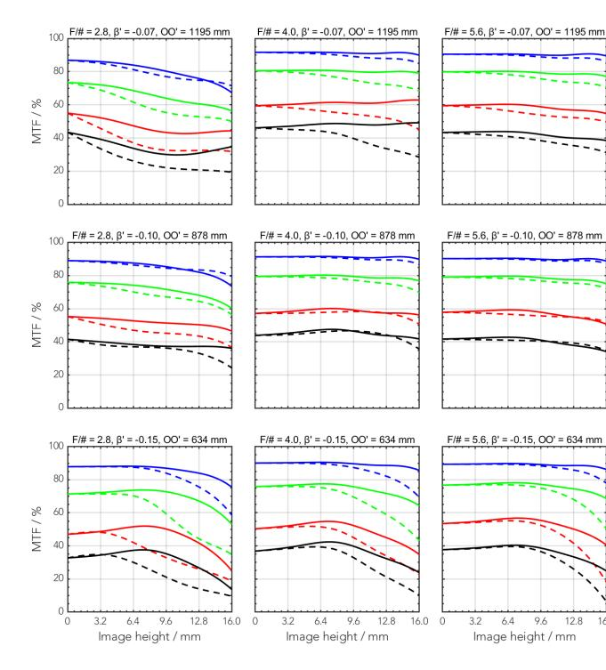
20 LP/mm, radial 40 LP/mm, radial --- 40 LP/mm, tangential --- 20 LP/mm, tangential
