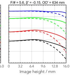
20 LP/mm, radial 40 LP/mm, radial — 80 LP/mm, radial – 120 LP/mm, radial --- 20 LP/mm, tangential --- 40 LP/mm, tangential --- 80 LP/mm, tangential --- 120 LP/mm, tangential
