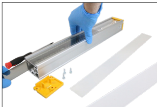
Insert the polarizer under the LD window
