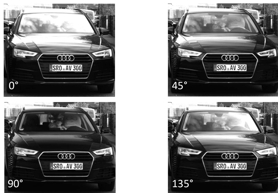
Figure 3: Polarization angle versus image brightness in sub-images
