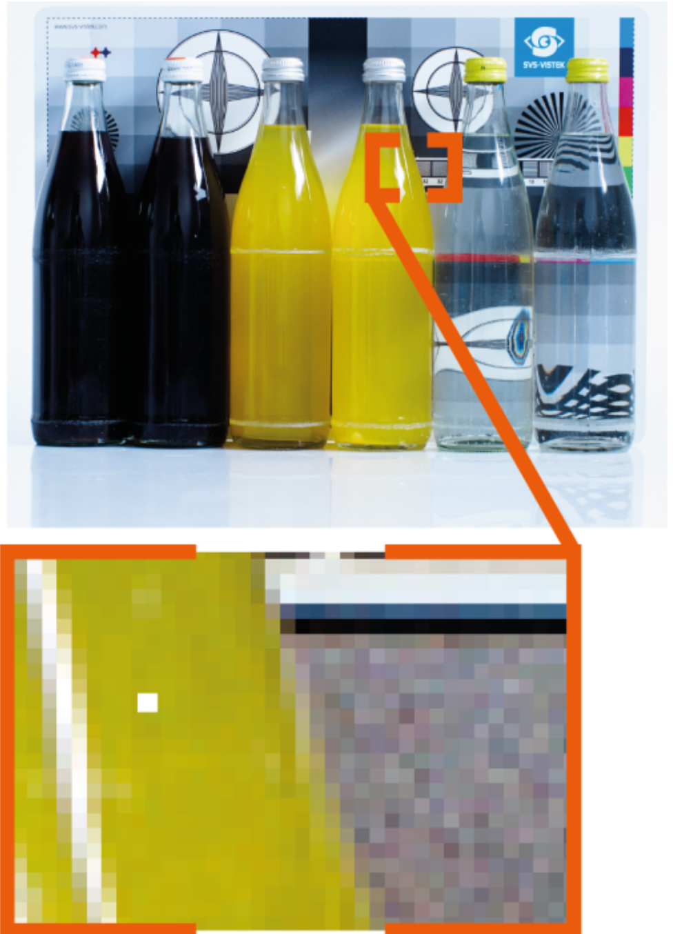
Fig. 5-23: Illustration of a defect pixel
