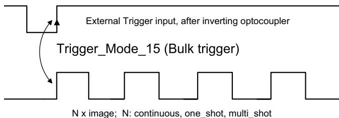
Figure 64: Trigger\_Mode\_15
