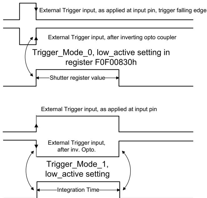
Figure 63: Trigger\_mode\_0 and 1
