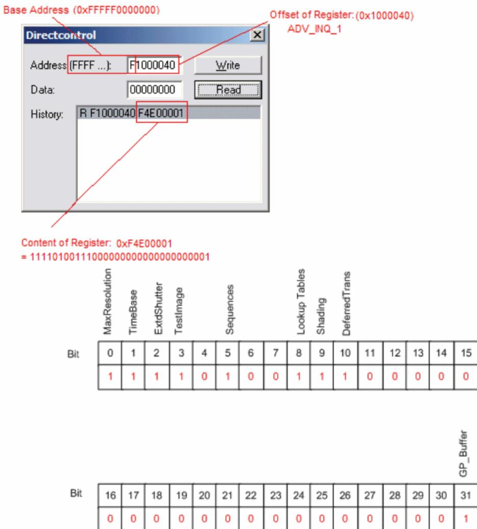
Figure 84: Configuration of the camera
