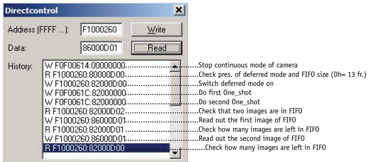
Figure 69: Example: Controlling deferred mode
