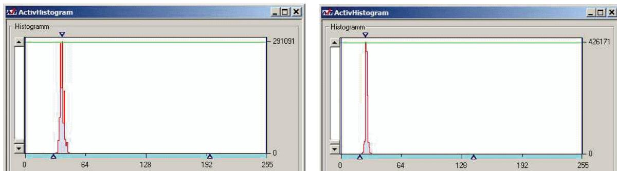
Figure 48: Effect of DSNU correction
