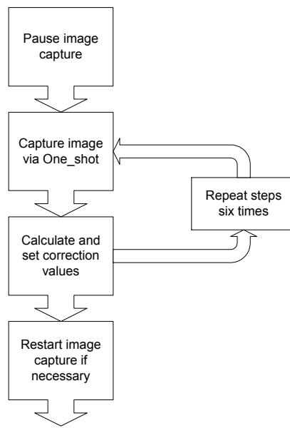
Figure 38: Automatic white balance sequence
