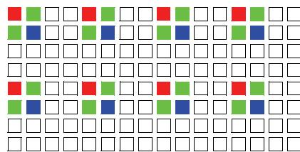
Figure 59: 2 out of 4 H+V sub-sampling (**color**)
