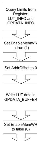
Figure 41: Loading an LUT
