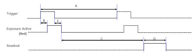
**Note**: Exposure Active in the figure above shows the waveform of the Red channel. The exposure timing delay for R, G, and B channels is 5.0us for each color (see below).
