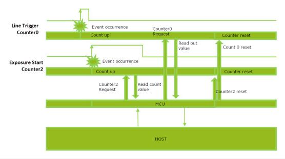
**Note:** You can reset a specific counter's count value by executing CounterReset[Counter0, Counter1, Counter2, Counter3, Counter4, Counter5].
