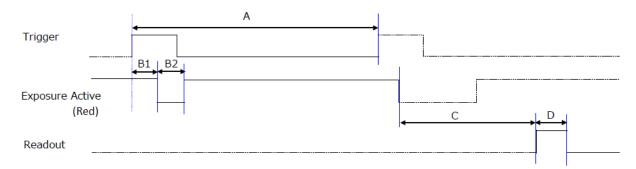
**Note**: Exposure Active in the figure above shows the waveform of the Red channel. The exposure timing delay for R, G, and B channels is 5.0us for each color (see below).
