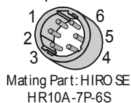
Figure 8: Hirose 6-pin Circular Male—Power Connector
