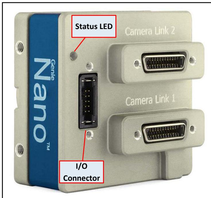
*Genie Nano-CL (medium casing) – Rear View*
