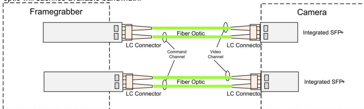
Figure 3. Linea ML Dual LC/SFP+ Connector Configuration
