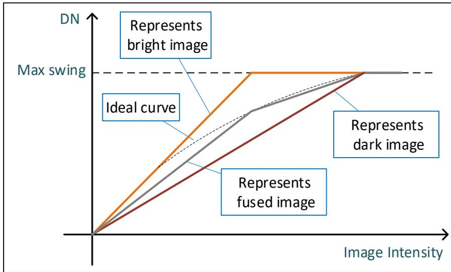
The HDR Demo mode demonstrates HDR imaging with a simple fusing algorithm,  $y = ax + b(1-x)$ , where  $0 < x < 1$ ,  $a$  and  $b$  represent dark and bright images, respectively.
