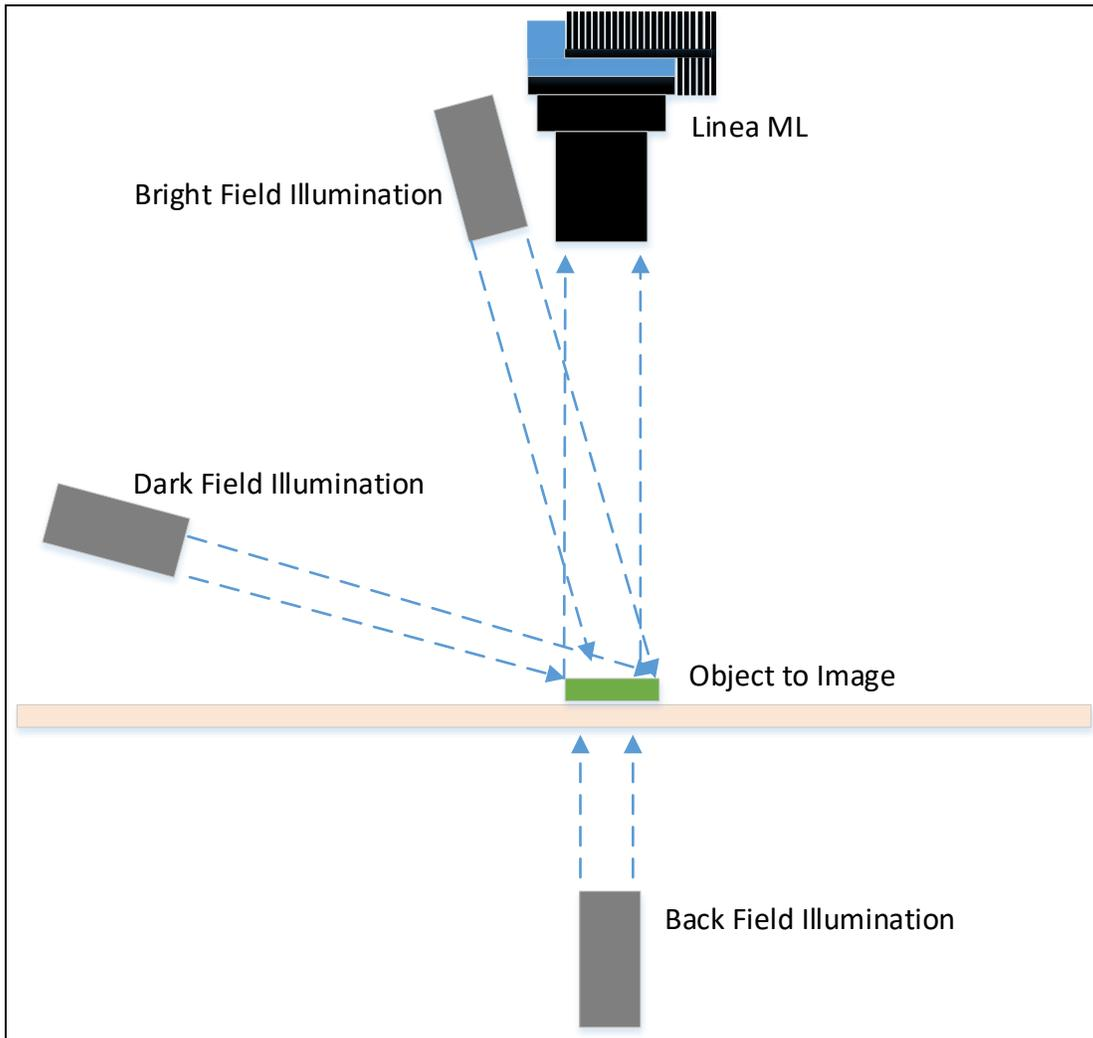
Figure 17. Typical Lighting Configuration
