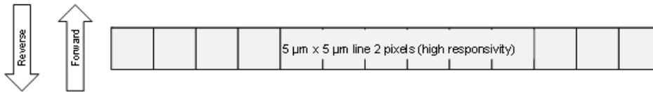
Figure 2: ML-FM-16K07A and ML-FM-16K15A Pixel Structure
