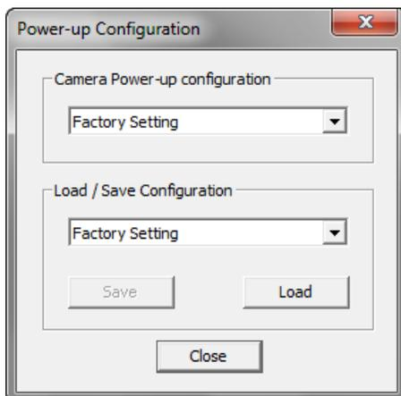
CamExpert provides a dialog box which combines the menu option used to select the camera's power-up state and the options for the user to save or load a camera state as a specific user set that is retained in the camera's non-volatile memory.
