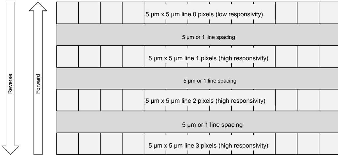
Figure 1: ML-FM-08K30H, ML-HM-08K30H and ML-HM-16K30H Pixel Structure
