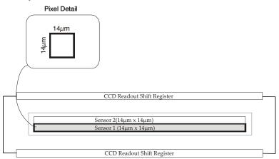
In low sensitivity mode, the camera uses a  $14\mu mx14\mu m$  pixel and captures the image using one sensor (Sensor 1).
