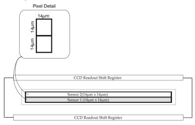
In high sensitivity mode, the camera uses a 14µmx14µm pixel and captures the same image twice, creating a brighter image.
