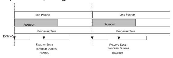
Mode 4: Smart EXSYNC, External Line Rate and Exposure Time
