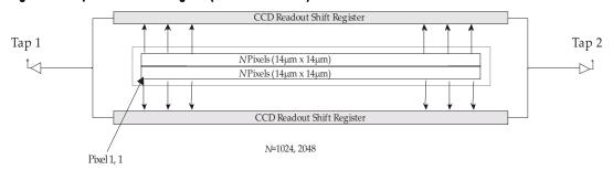
Figure 2: 1 Tap Sensor Block Diagram (01K40 and 02K40)
