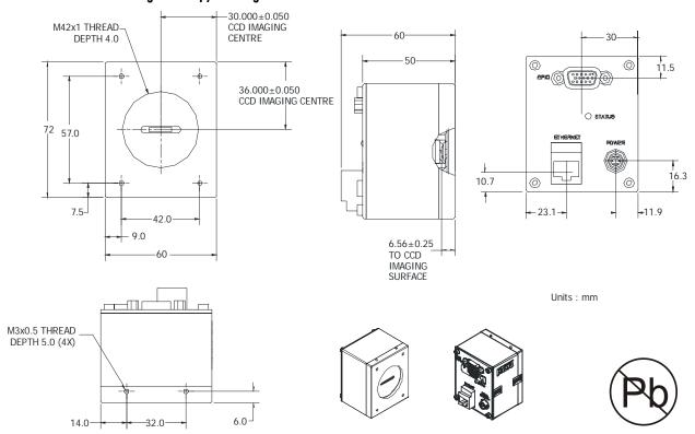
Figure 18: Spyder 3 GigE Heatsink Mechanical Dimensions
