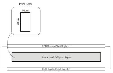
In tall pixel mode, the camera uses a  $28\mu$ mx $14\mu$ m pixel and captures an image two times taller than in high or low sensitivity mode, creating a taller image.
